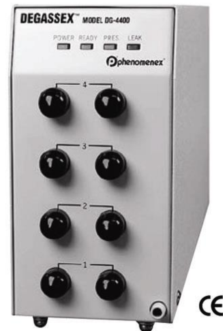
Degassing four solvents
