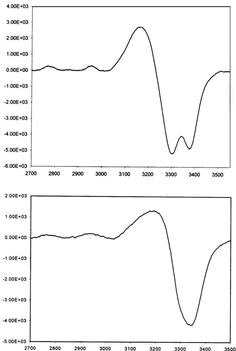
Fig. 9. EPR spectra of a four-coordinate complex  $[\text{Cu}(\text{L1})](\text{ClO}_4)_2$  (top) and a five-coordinate complex  $[\text{Cu}(\text{L3})](\text{PF}_6)_2$  (bottom) measured in  $\text{CH}_3\text{CN}$  frozen glass (77 K).
