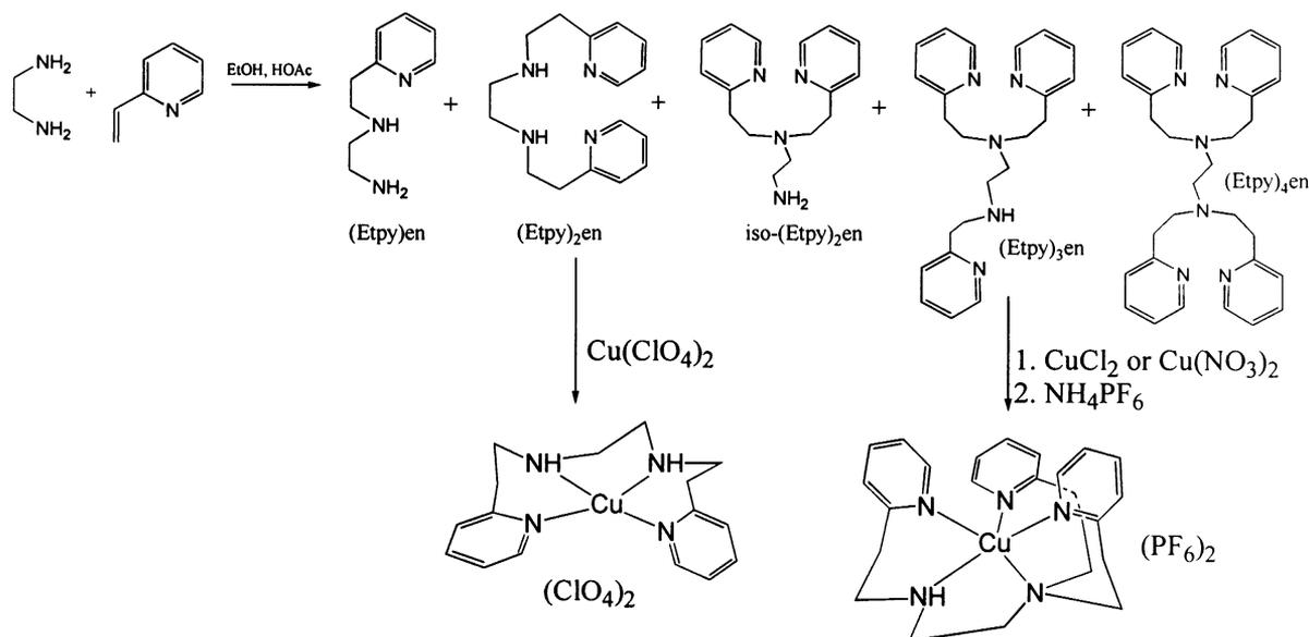
Fig. 3. Synthesis and isolation of the copper(II) complexes with tetra- and pentadentate aminopyridine ligands bearing ethylpyridine pendant arms.
