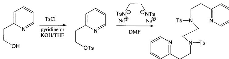
Fig. 2. Synthesis of the tosylated tetradentate ligand (Etpy)<sub>2</sub>Ts<sub>2</sub>en (L2).
