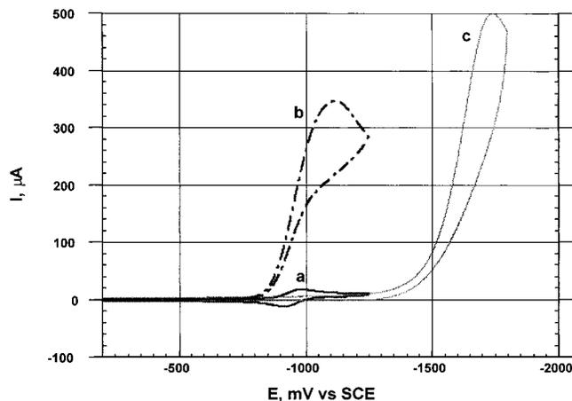
**Figure 6.** Cyclic voltammograms on pyrolytic graphite disk electrodes at  $50 \text{ mV s}^{-1}$  in  $0.2 \text{ M TBAB}$  in DMF of (a)  $1 \text{ mM}$  complex  $[\text{NiL2}]^{2+}$  alone, (b)  $1 \text{ mM}$  complex  $[\text{NiL2}]^{2+} + 12 \text{ mM}$  1,2-*trans*-dibromocyclohexane, and (c)  $13 \text{ mM}$  1,2-*trans*-dibromocyclohexane alone.
