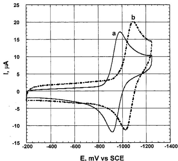
**Figure 5.** Cyclic voltammograms on pyrolytic graphite disk electrodes at 50 mV s<sup>-1</sup> in 0.2 M TBAB in DMF: (a) 1 mM complex [NiL2]<sup>2+</sup> and (b) 1 mM complex [NiL1]<sup>2+</sup>.
