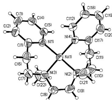
**Figure 2.** ORTEP drawing of complex cation [NiL3]<sup>2+</sup>. Selected bond lengths (Å) and angles (deg): Ni(1)–N(1), 1.892(2); Ni(1)–N(2), 1.949(2); Ni(1)–N(3), 1.927(3); Ni(1)–N(4), 1.907(2); N(1)–Ni(1)–N(4), 91.35(10); N(2)–Ni(1)–N(4), 90.25(10); N(2)–Ni(1)–N(3), 87.89(11); N(1)–Ni(1)–N(3), 90.63(10).
