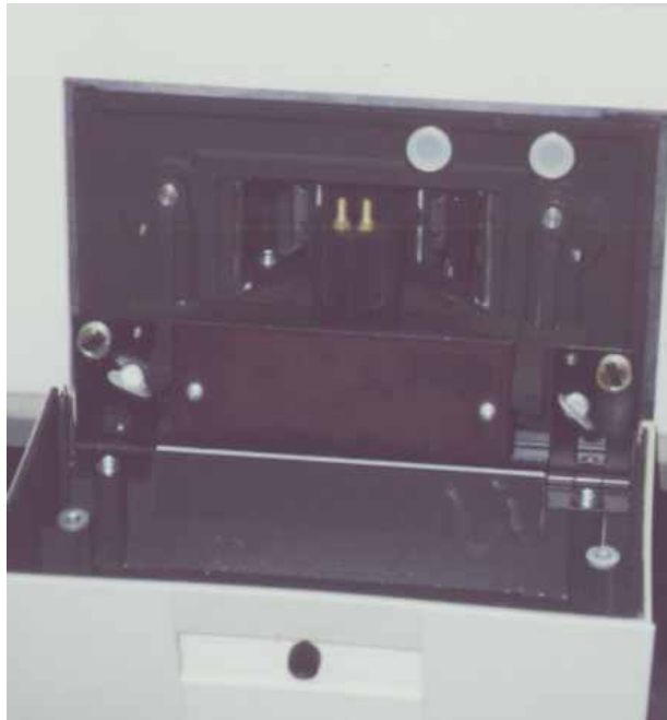
Sample compartment of PerkinElmer LS-55 spectrofluorimeter
